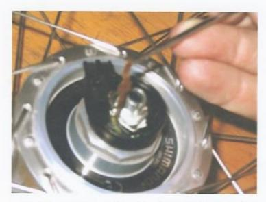
You'll notice an opening on the bottom of the plug assembly body. This opening is large enough for the current connector to pass though, Carefully work the plug assembly body off the buth.
