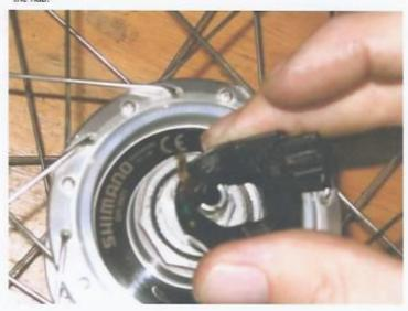
If this is the first time your hub has been opened, there will be a mess of white, semi-solid substance (which I assume is Teflon) slathered around the wire where it passes through an opening in the silver metal spacer at the triangular end. You'll probably need to pick away some of the Teflon to remove the spacers. Below the spacers, the wire runs in the groove on the hub axle. After you've removed the spacers (parts 4 and 5), the hub will look like this:
