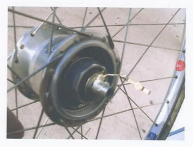
Place the wire along the groove in the hub so that the back plate (part 3) can be removed and the cone screwed off the axie without damaging the wire.
