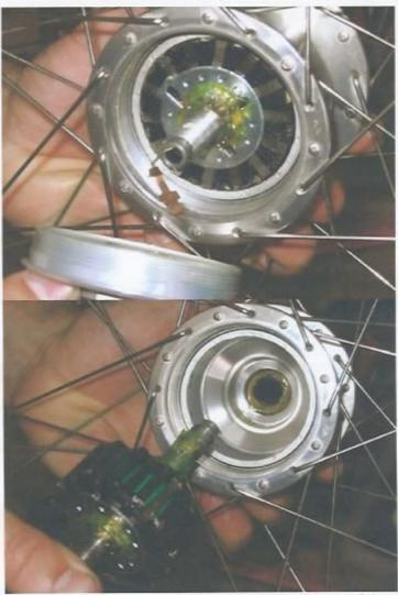
With the axle cut of the way, the bearings on each side of the hub can easily be removed and the cups cleaned and inspected. Remove all the old grease and repack, replacing bearings as necessary.
